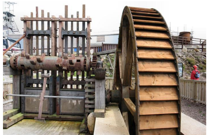
Eight heads of Cornish stamps powered by a waterwheel
