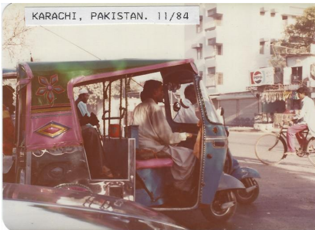
A common mode of transportation in Pakistan. Three wheeled scooters with two-cycle engines. They are also popular in India.
