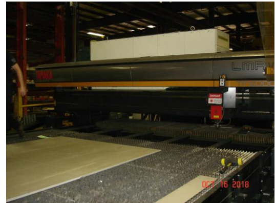
6,000 W Laser cutter. The table can handle plates 13' x 80"
