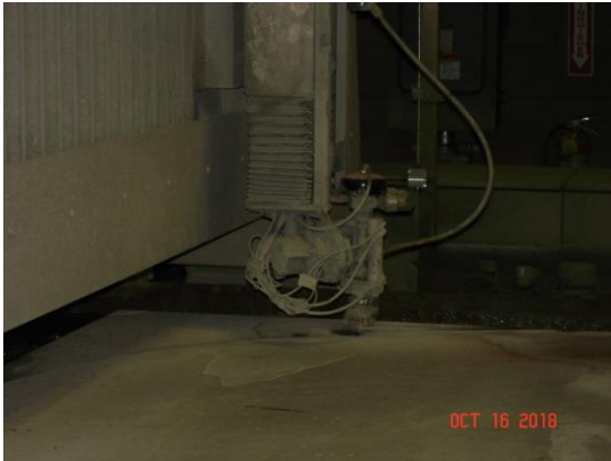
Water jet cutter, at 80,000 psi
