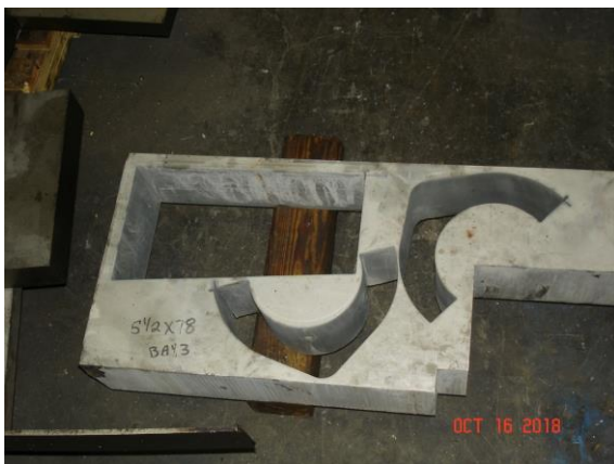
Water jet cut. Note the sharp edges and smooth cut
