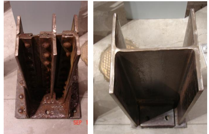
Fabricated beam - Bethlehem Steel Wide-Flange "H" beam
