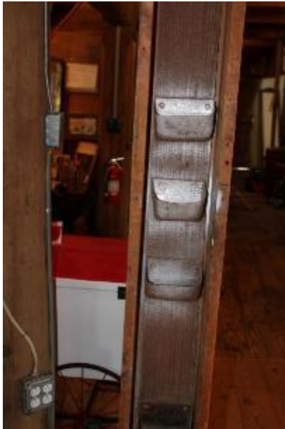
Bucket elevator; the buckets are 4" wide attached to a canvas belt
