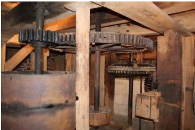
Wooden gear teeth. If there is a jam, the easily replaceable teeth will break.
