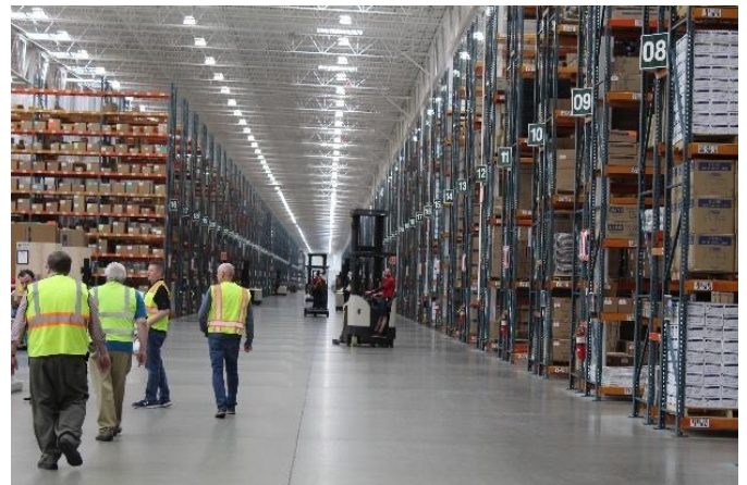
Center aisle. Note battery powered Reach Trucks and Stock Pickers, for transporting products. Internally, the hallway appears to be a half mile long!
