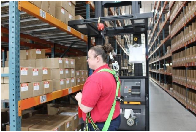
Safety is of primary concern. Each operator wears a safety harness.
